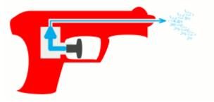
actually putting pressure on the water—and that's why it squirts out at a much higher speed than you move the trigger. If water weren't incompressible, water pistols wouldn't work properly. You'd squeeze the trigger and the water inside would simply squash up into a smaller space—it wouldn't shoot out of the nozzle as you'd expect.
